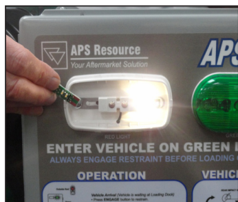
Inside LED Upgrade
